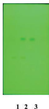
**Figure 1.** Developed TLC plate of showing separation of BER and GZ at  $R_f$  value of  $0.40 \pm 0.02$  and  $0.68 \pm 0.02$ , respectively (Track 1 – Standard solution of BER, Track 2 – Mixture of BER and GZ, Track 3 – Standard solution of GZ)
