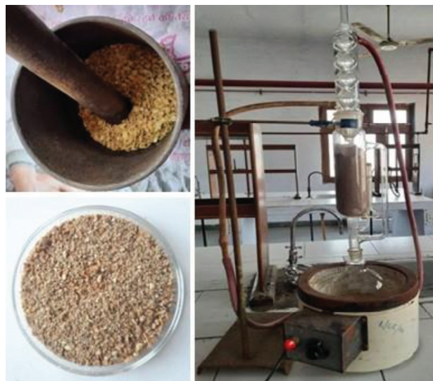
Figure 1: Putranjiva roxburghii Wall. Crushed Seeds and Soxhlet Extraction Process
